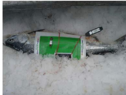
Icicle Seafood uses Infratab's RFID tags to track temperature readings for fish throughout the supply chain.
